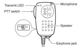
The HM-75LS has a lock switch on the backside to prevent accidental frequency changes, and so on.
