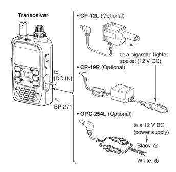
**NOTE:** Up to 5 W (approximately) of maximum output power is possible when using external DC power. However, when the supply voltage exceeds 14 V, the built-in protection circuit activates to reduce the transmit output power to approximately 2.5 W.
