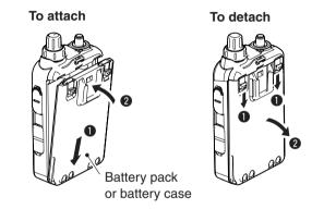
Even when the transceiver power is OFF, a small current still flows in the radio. Remove the battery pack or case from the transceiver when not using it for a long time. Otherwise, the battery pack or installed batteries will become exhausted.
