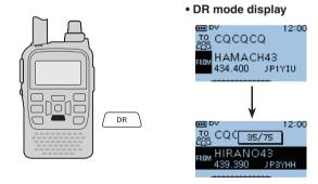
② Rotate [DIAL] to select a desired access repeater.
