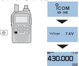
The opening message and power source voltage display options can be turned ON or OFF in the DISPLAY menu.
