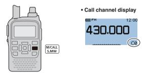
② Rotate [DIAL] to select a desired Call channel.
